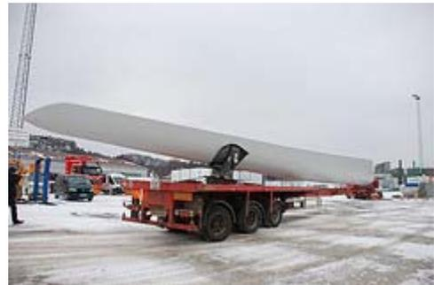
One manufacturer overcoming the size and weight challenges is Enercon. Their 63 meter blades for 7.5 MW E-126 turbines are some of the longest in the market today. To take the edge off the length problem, Enercon designed the blades to fold in half for transport. They are then delivered in sections and commissioned on site.<sup>iv</sup>
